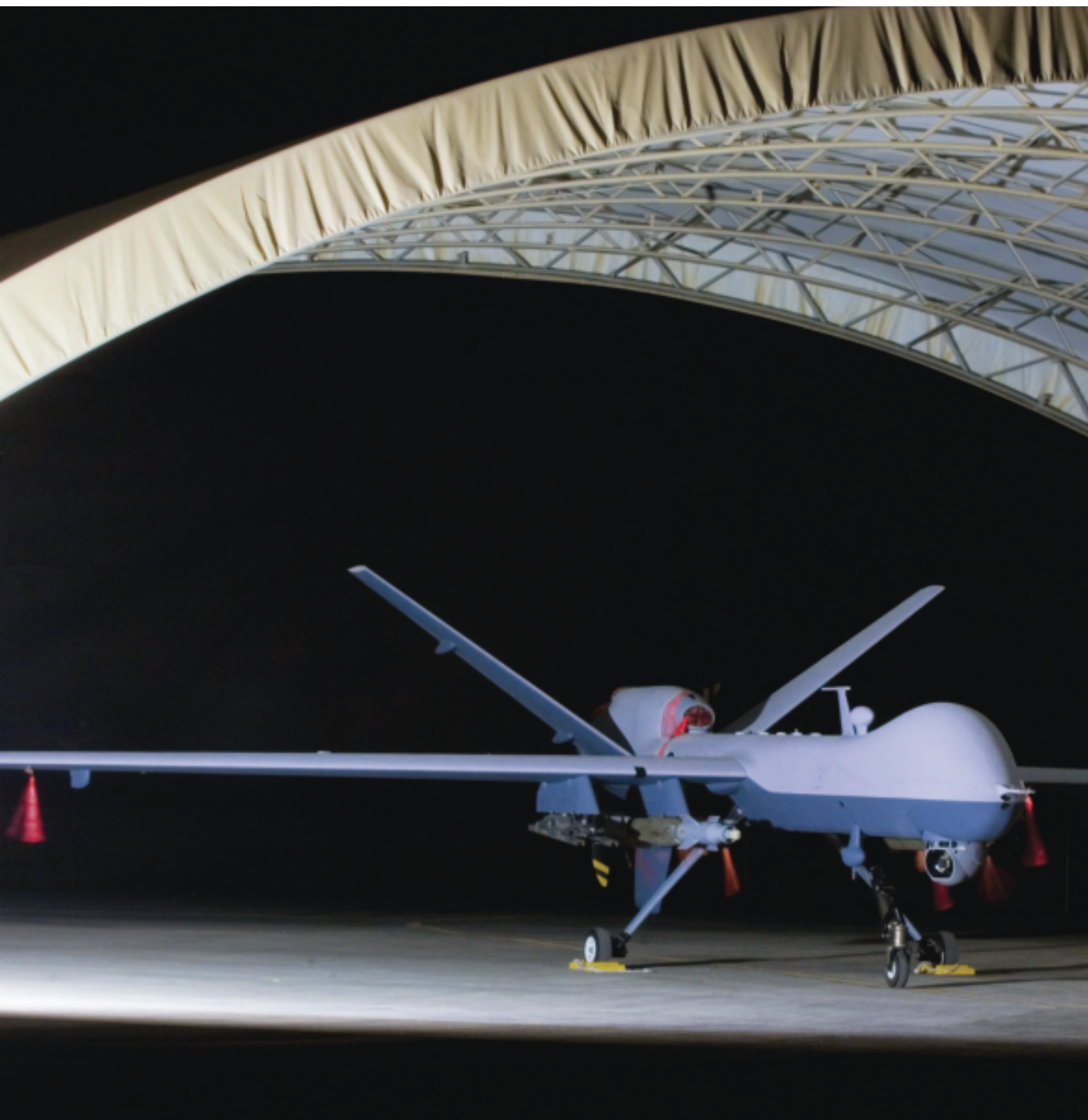
An armed MQ-9 Reaper unmanned aircraft sits in a shelter Oct. 15 at Joint Base Balad, Iraq, before a mission. Larger and more powerful than the MQ-1 Predator, the Reaper can carry up to 3,750 pounds of laser-guided bombs and Hellfire missiles.
